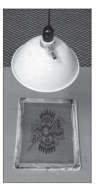
to be filled in, paint a little of the sensitized emulsion onto the screen, let dry in the dark as before, and then expose to light. Let the screen cure for a bit in the sun or under a light until it dries.
