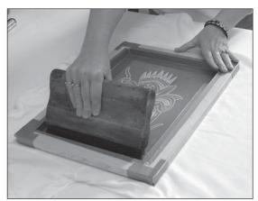
c. Holding the squeegee at a 45 degree angle, pull the line of ink across the image. It may take a little experimenting to find the correct amount of pressure when screening the ink. You may want to have
