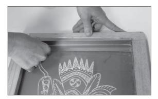
a. Taping will help prevent ink from leaking through the areas where the screen fabric and the wood frame meet while printing. This will help to keep the edges of your print clean. On the inside of the screen, fold the tape in half lengthwise and place half of the tape on the screen and half on the wood frame. Continue all along the inside of the frame.
